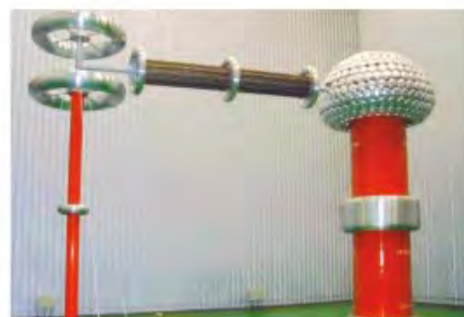
1000kV Power Frequency Test Transformer
