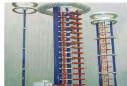
3000kV Lightning Impulse Voltage Generator
