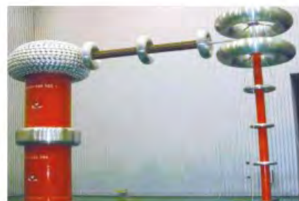
600kV Power Frequency Test Transformer
