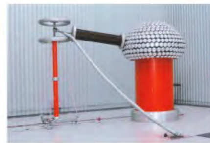
300kV Power Frequency Test Transformer
